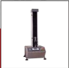
Universal Tensile Testing Machine (UTM)
